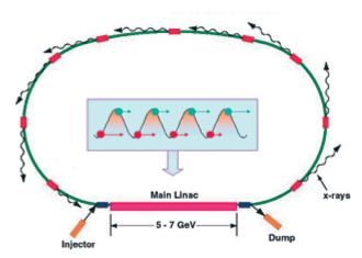
In the proposed Energy Recovery Linac facility, electrons are pushed to almost the speed of light, "surfing" on the crest of microwaves in a linear accelerator (linac). The accelerated electrons make one trip around the Cornell Electron Storage Ring (CESR), and returning electrons feed back into the linac and give up their remaining energy to the microwaves. When the full-scale facility is built, the 1.3 kilometer-long linac will occupy a tunnel underneath campus parking lots.
