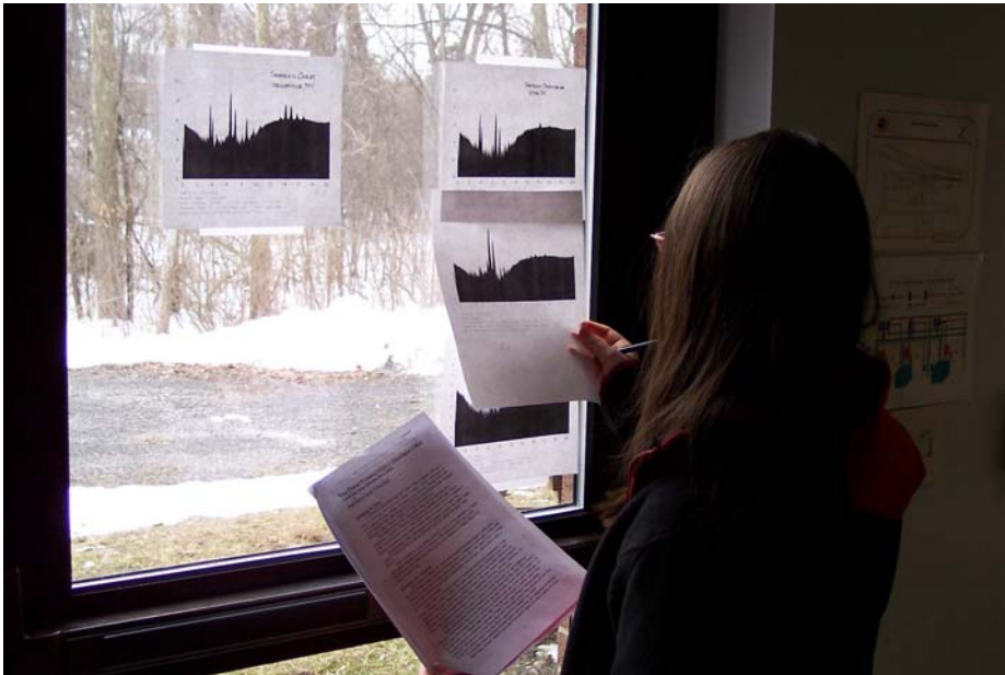
Using sunlight shining through an outside window, a student tries to overlay and match her x-ray fluorescence spectrum to those from known samples.
