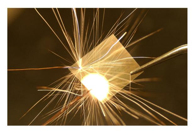
A thin foil multilayer, with alternating aluminum and nickel layers, releases heat and light as the layers react to form a metallic compound. At the CHESS A2 station small x-ray beams focused by a tapered glass capillary records the structure of the compound as the reaction front moves across the foil. [**Photograph by:** Maximilian Franz courtesy of Reactive NanoTechnologies (RNT). From the Hufnagel and Weihs groups at Johns Hopkins University]
