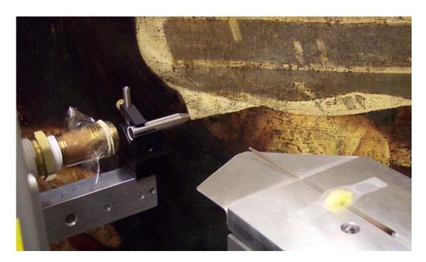
Shown at right is a tapered glass capillary optic used to focus x-ray beams down to 10 microns or so in size. The input end is stained brown by long-term x-ray damage to the glass. This optic was fabricated by graduate student Sterling Cornaby and is pictured in use to focus a small x-ray beam onto an oil painting. Confocal x-ray fluorescence mapping is used to examine buried paint layers.
