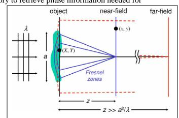
Illustration of coherent x-ray wave propagation with a distorted object approach both for the near-field Fresnel diffraction, where an object extends into multiple Fresnel zones solid lines and for the far-field Fraunhofer diffraction, where an object occupies only the center of the first Fresnel zone dashed lines.
