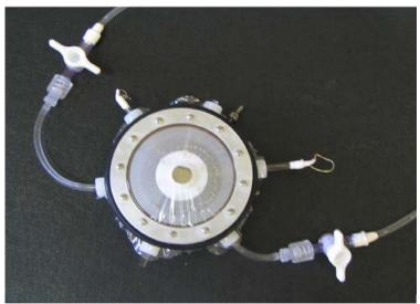
Figure 2. Electrochemical cell for *in-situ* X-ray characterization of catalyst surfaces. (Abruña group).
